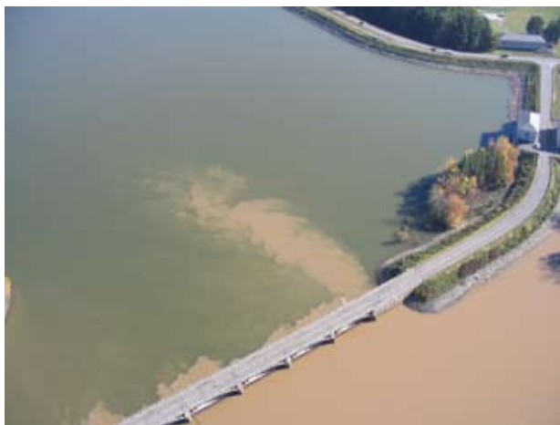
Heavy rain can cause sediments to become suspended in water, reducing its quality, as seen in the brown swath above in New York City's Ashokan reservoir following Hurricane Floyd in September 1999.
