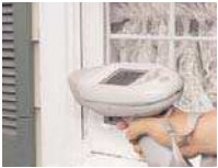
NITON's XLp 300 Series Lead Analyzer, pictured above, can measure the concentration of lead in paint even when covered by 50 or more layers of non-lead paint of unknown thickness and composition.
