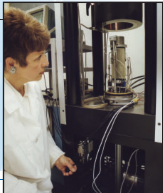
The GHASTLI system simulates deep-sea conditions.
