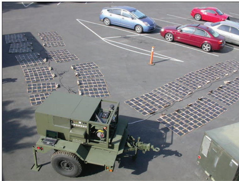
Figure 5: Deployable Renewable Energy Alternative Module Prototype
