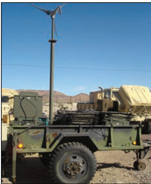
Figure 14: Transportable Hybrid Electric Power Stations (THEPS)
