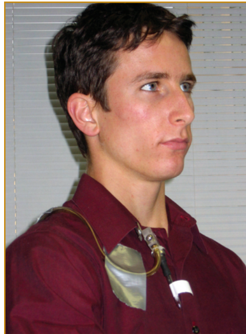
Figure 8: Attach the pump to a belt at the employee's hip. Insert the sorbent tube in a commercially available tube holder or similar device and clip it in the area of the employee's lapel, with the sorbent tube hanging down.
