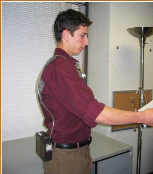
Employee wearing an air sampling pump and sorbent tube.
