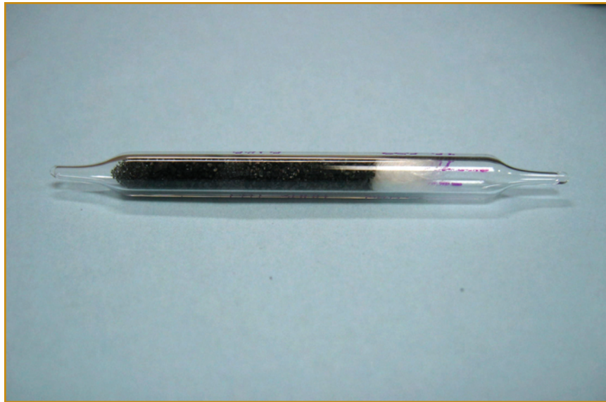
Figure 2: Communicate with the analytical laboratory to select an appropriate sorbent tube for the situation to be monitored. Sorbent tubes come in several sizes, which may appear similar to, but not necessarily identical to the tube shown here.
