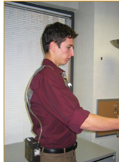
Figure 9: Air sampling professionals often use duct tape to hold excess plastic tubing in place so that it will not get in the employee's way. Provide adequate slack in the plastic tubing to allow the employee to reach and bend. For each sorbent tube used, enter on the sampling form the time that sampling starts with that tube. Turn the pump ON and check periodically to be sure that it is running smoothly. Use a fully charged pump battery to ensure that the pump will run for the full sampling period.
