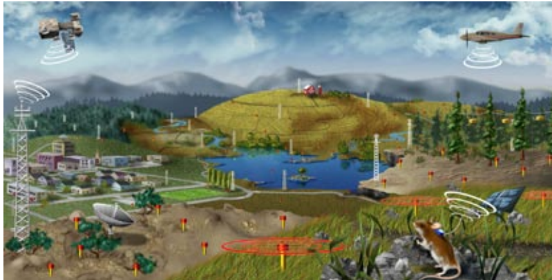
This illustration depicts how infrastructure platforms that comprise the NEON sensing system will be deployed across the landscape in wildland, managed, and urban environments. BioSensor Towers, sensor networks, radar, mobile sensing, remote sensing, experimental facilities, education facilities, and forecasting facilities will be networked by leading-edge cyberinfrastructure into a national research platform.
