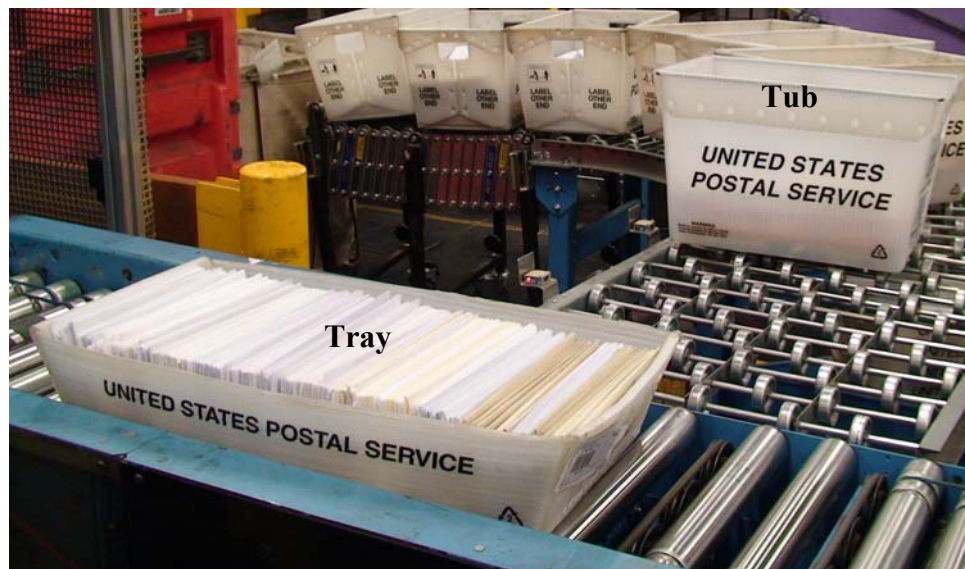
Figure 6. Examples of tubs and trays used to distribute mail through the P&DC
