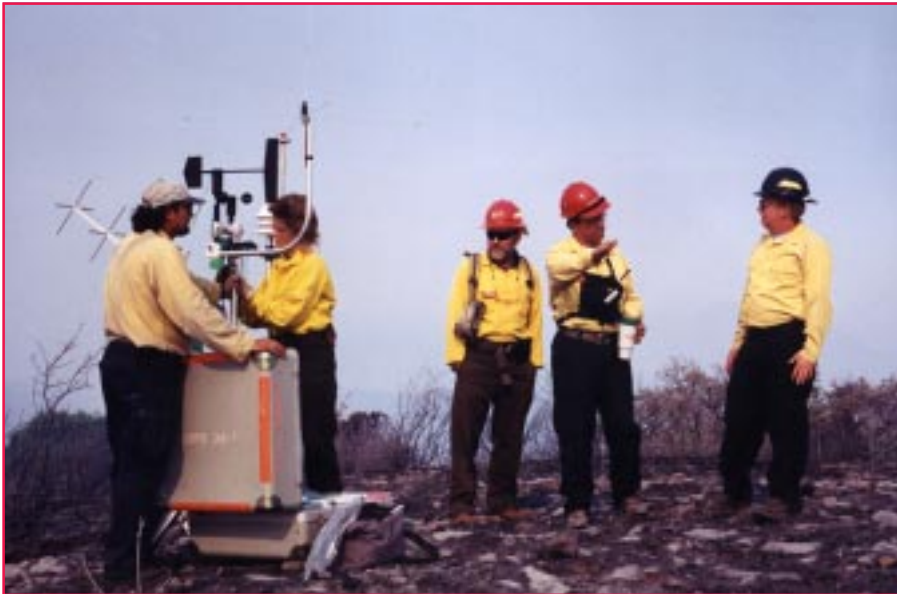
Technical specialists replace a burned-over NIFC FIRE Remote Automated Weather Station (RAWS) on the Bircher Fire. To the right of the RAWS, local fire managers talk to a fire behavior analyst. Photo: Charles S. Maxwell, National Weather Service, Albuquerque, NM, 2000.
