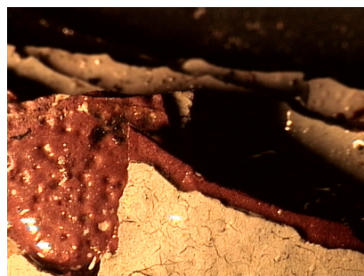
Under the microscope in the lab, it was determined that this piece of suspected debris is a small piece of metal, with layers of paint.
