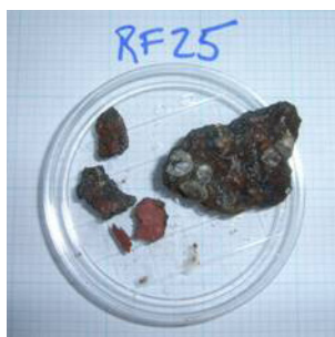
Both metal debris and a paint chip were found in this surface sediment sample collected in the reserve fleet area.
