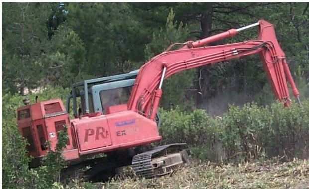
PG&E used this brush mower in the park to maintain their lines.
