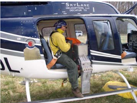
A PSD or “ping-pong ball machine” is loaded in preparation for aerial ignition at Kings Mountain National Military Park
