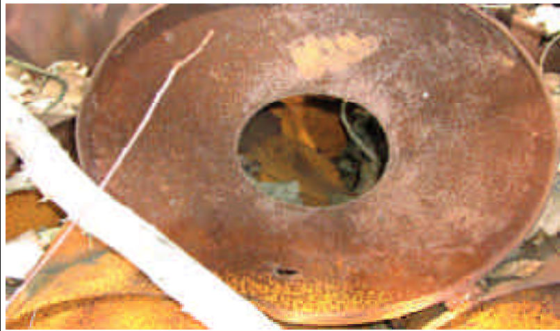
Figure 4. Close up view of a hole in one of the 128 drums located in Wetland 1
