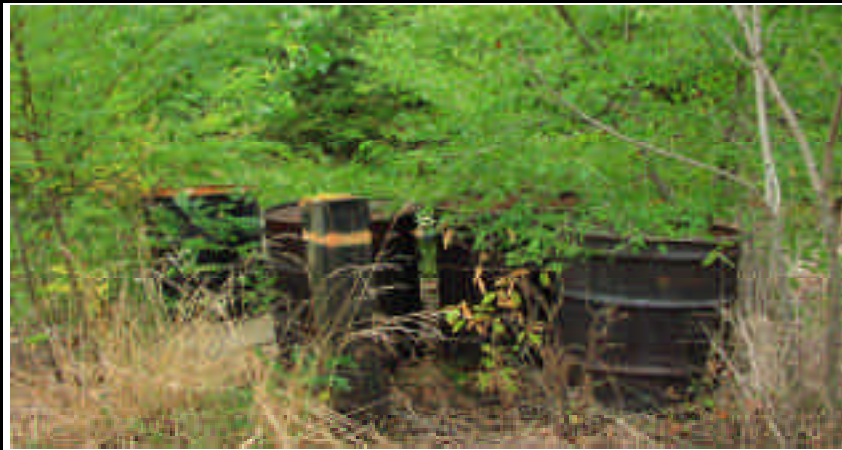
Figure 9. Four drums located near MW-7 containing either soil cuttings or purge water from wells
