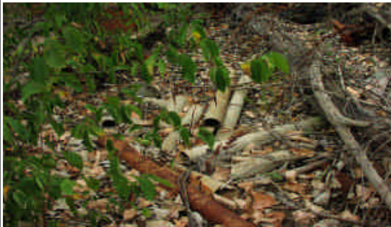
Figure 5. Pile of tan colored pipes containing asbestos
