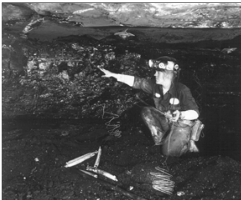
Charging bore holes in the coal face of a deep mine in Western Kentucky, owned and operated by Pyro Mining Co.
