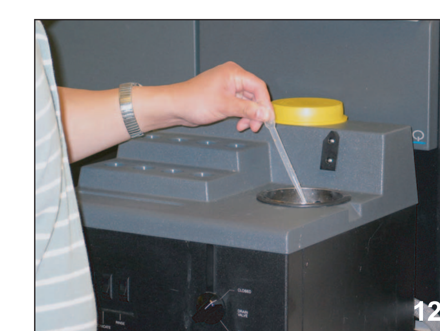
After splitting, the cores were subsampled at various intervals for grain size, water and organic content, mercury and methylmercury concentration, and geochronology (to be reported separately). Figure 12 (left) shows a technician placing a prepared grain-size subsample into the laser particle-size analyzer. Some of the results of this analysis are shown in the sediment sections on Figure 5.
