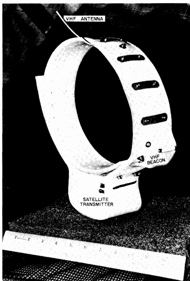
Fig. 24. Third-generation transmitter built by Telonics, Inc. This particular platform transmitter terminal (PTT) is configured for a polar bear and weighs 2 kg.
