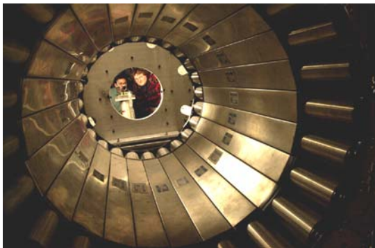
Internal view of new Germanium gamma ray detector array for study of structure of radioactive ions
