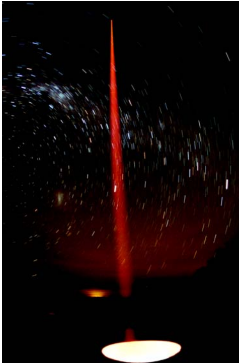
Sodium laser tests from Cerro Tololo Inter-American Observatory. These tests are part of a joint effort by Gemini, CTIO and ESO to characterize the seasonal variations in the atmospheric sodium layer in preparation for adaptive optics laser guide star systems like Gemini's Altair and the planned Multi-Conjugate system currently being designed by Gemini.
