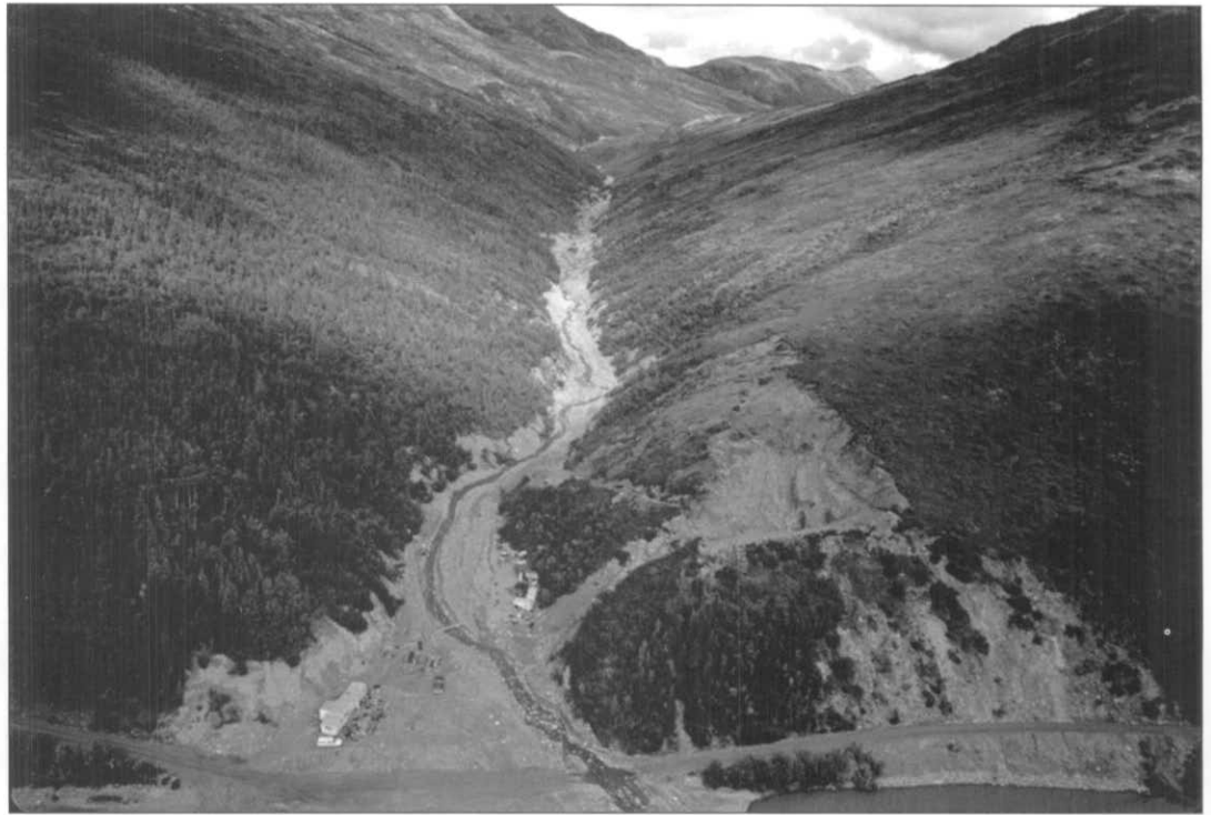
Eureka Creek, originally staked in 1905, had intermittent placer mining occurring at its mouth and along the entire length of the creek until 1985. This photograph shows the park road crossing at Eureka Creek and mining activities shortly before the 1985 mining injunction, including a recent bench cut on the right. NPS Photo
