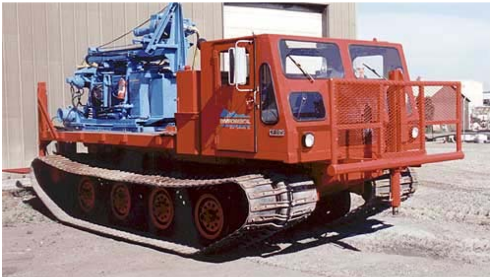
FIGURE 6 – NODWELL 110 ATV CARRYING A LIMITED ACCESS DRILL
