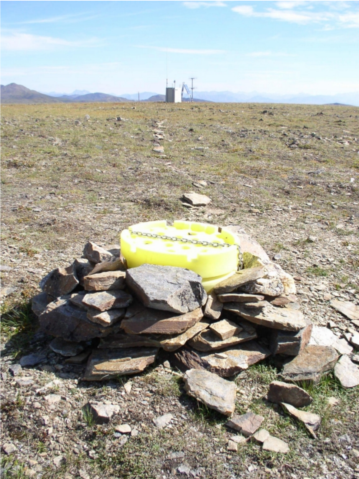
Figure 2.4. Example of seismic drum and buried cable to equipment hut.
