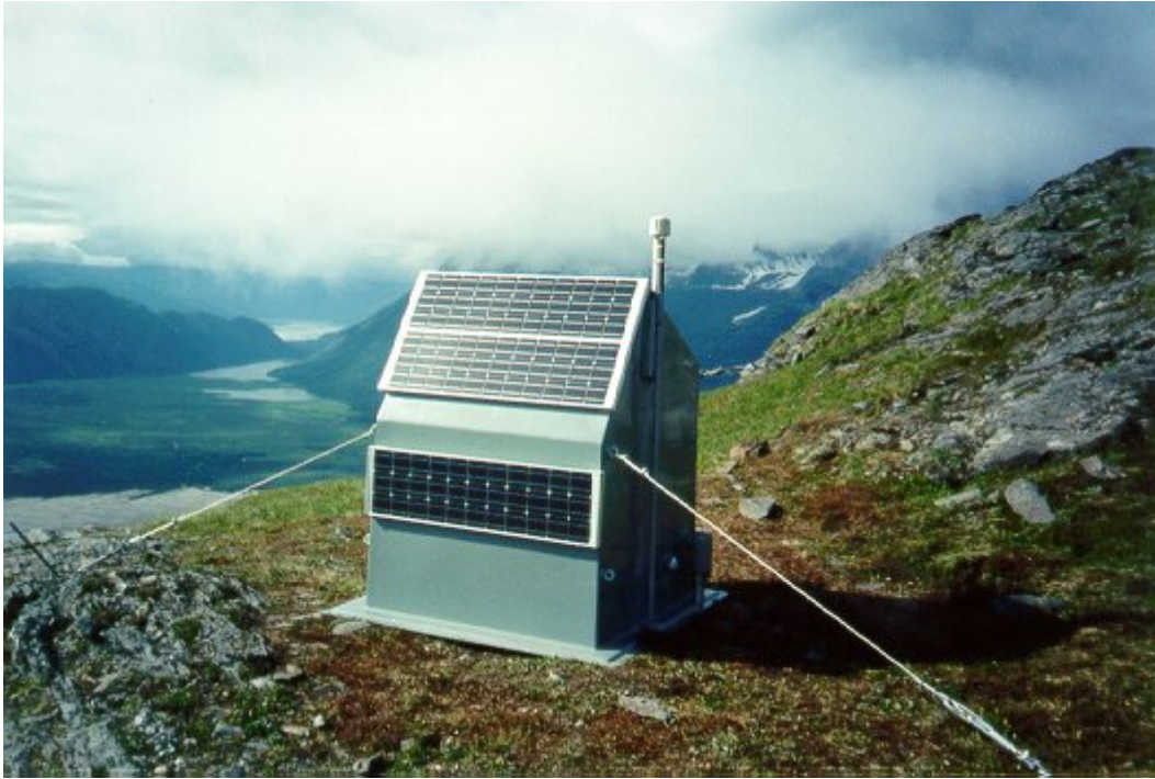
Figure 2.2. Typical fiberglass seismic hut, same as is proposed for the Castle Rocks installation. Solar panels provide power, guy wires prevent movement. Door is on opposite side. Hut is 16 square feet (4'x4'), 5 feet high, and gray to limit visibility.
