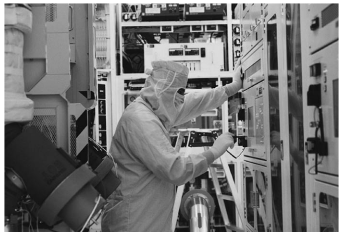
Semiconductor processors wear protective garments called “bunny suits” to avoid contaminating the chips they produce.
