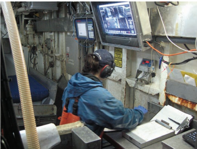
Observer sampling station on Amendment 80 F/V Seafisher. Shows flowscale, table and platform scale, video monitoring display, and display for platform scale.
