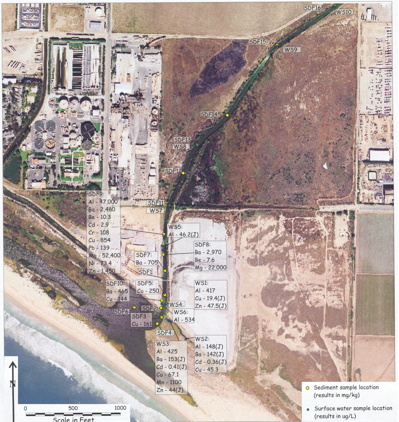
Figure B4. Surface Water Sample Locations Along the Oxnard Industrial Drain, Halaco Site, Oxnard, California
