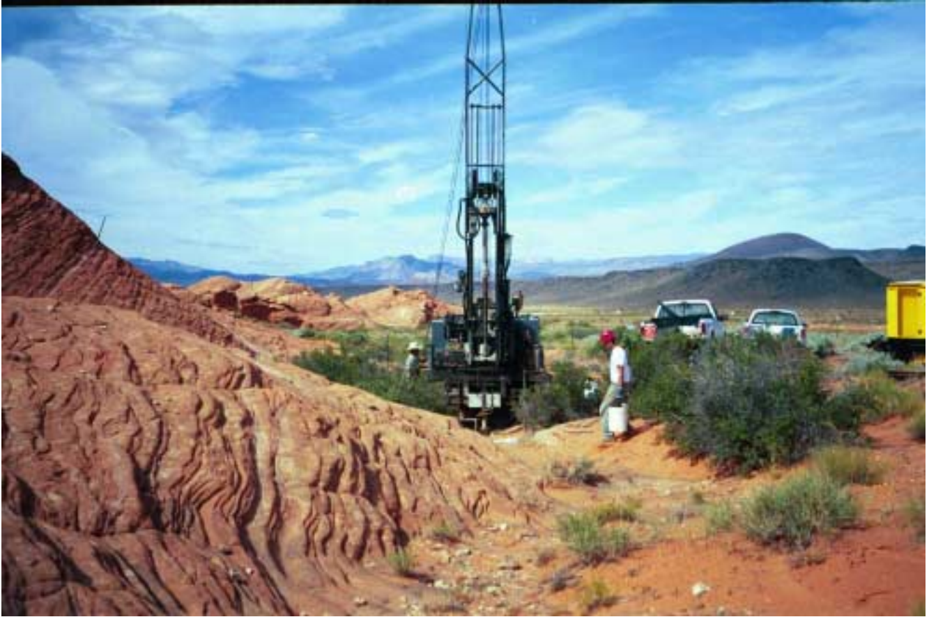
Collecting core samples at Sand Hollow basin, Utah, for evaluating natural recharge.
