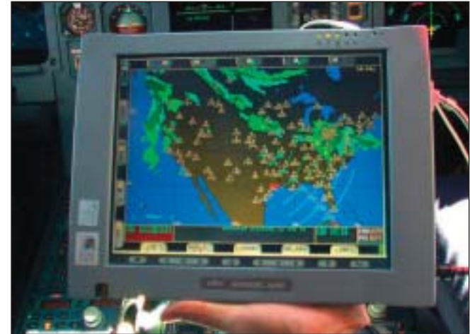
NASA's graphical cockpit weather displays improve aviation safety and on-time performance. They provide aircrews with real-time information that will allow them to avoid areas of hazardous weather and turbulence.
