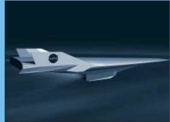
The X-43 scramjet hypersonic demonstrator represents the intersection of air and space transportation, potentially serving as a first stage to orbit, or as a means of global reach for military applications.
