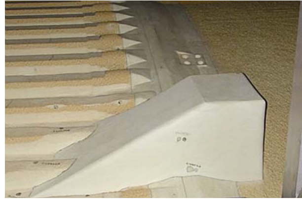
Figure 3.2-1-2. ET forward bipod ramp (foam).
