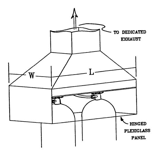
Figure 18. The recommended cylinder hood design features a hinged Plexiglas panel which can be raised to remove the empty cylinder and slide in the new cylinder. In the down position, the panel protects the worker's face from spray while allowing the worker to see the connection point while the empty cylinder is being disconnected and then the new cylinder is connected to the supply line.
