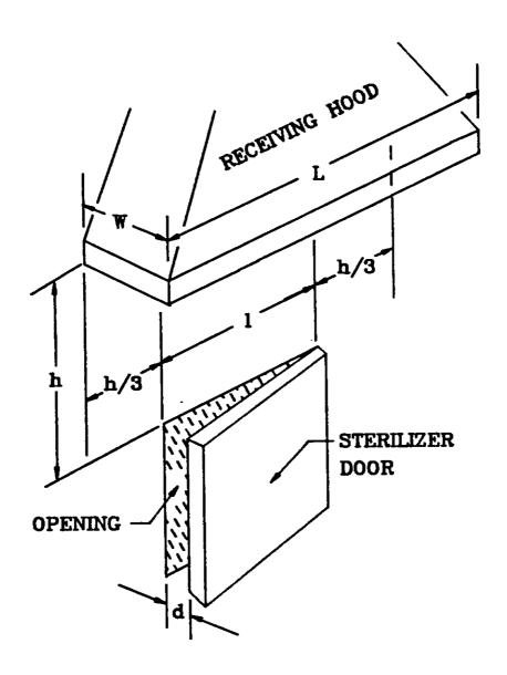
Figure 17. A canopy hood above the sterilizer door can be used to exhaust the EtO which rises in front of the sterilizer during the door-cracked period. (See text for a discussion of the appropriate values for the variables.)
