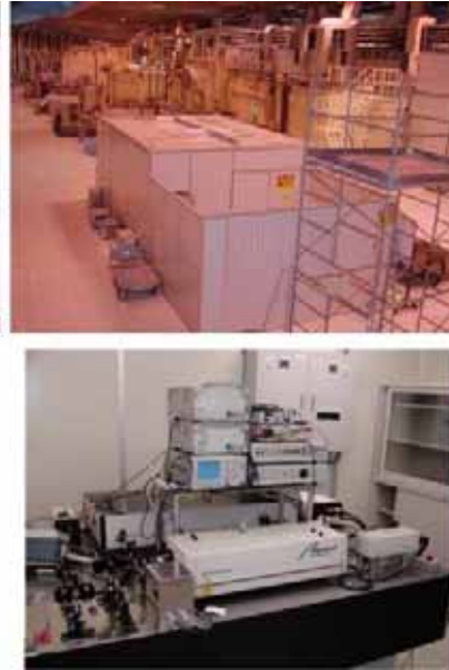
② BL19LXU 27m-long undulator Soft x-ray beamline
