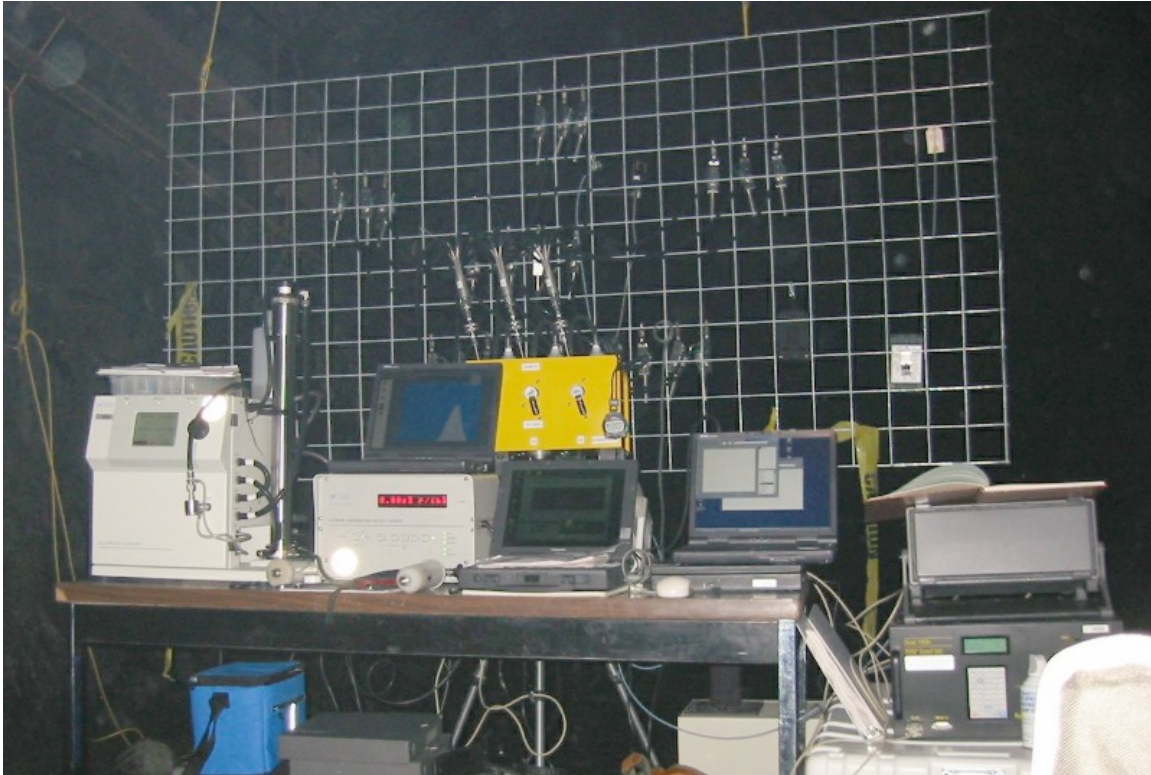
Figure 13.—Downstream sampling station showing instrumentation and grid supporting DPM samplers, anemometer, and iTX gas monitor.
