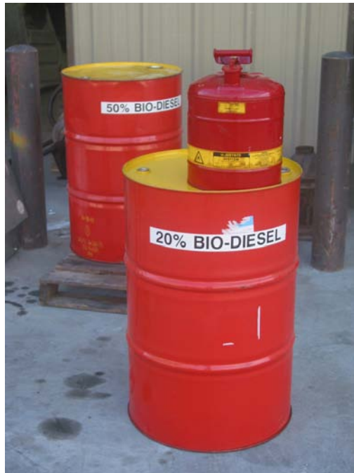
Figure 7.—Mixing and storage vessels for B20 and B50 biodiesel #2 diesel fuel blends.
