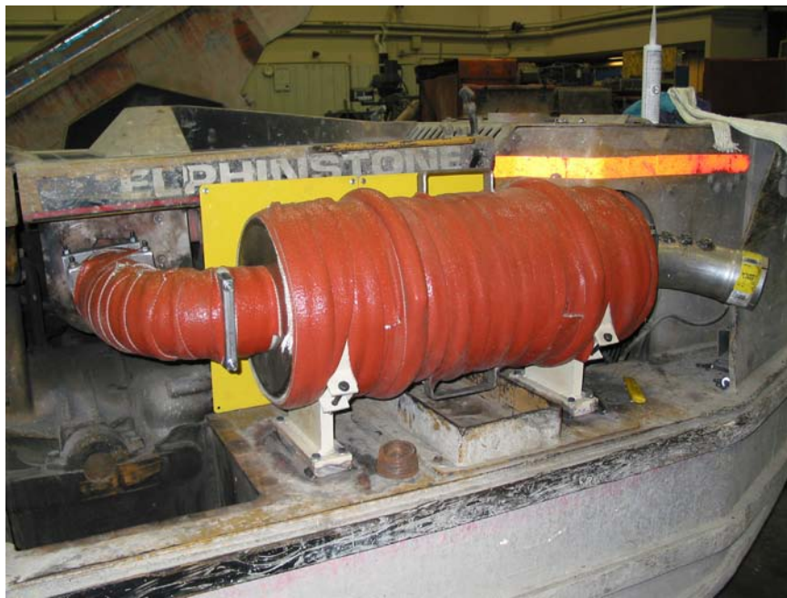
Figure 5.—ECS Cattrap DPF system on LHD #92526.
