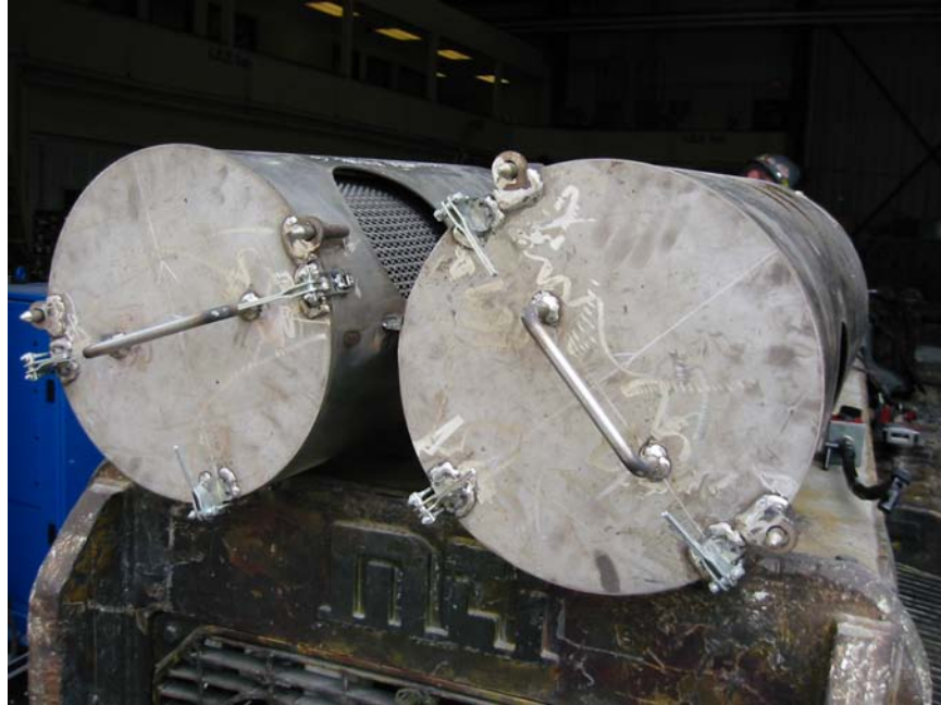
Figure 4.—Mac's Mining Repair filtration system on LHD #92506 used for testing Donaldson P604516 and Filter Services DFEs.
