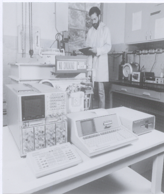
Figure 3.—Frictional ignition chamber with oscilloscope and microcomputer analyzing system for determining radial and tangential impact forces.
