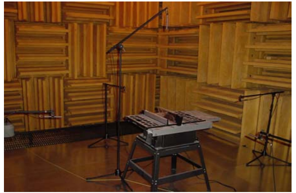
Sound power level of a table saw being measured in a semi-anechoic environment.
