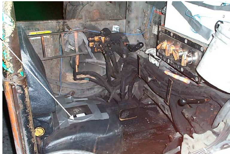
Figure 8.—Instrument setup on the mid-coal-seam shuttle car seat.
