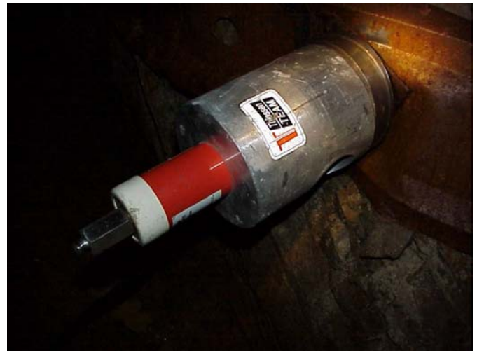
Figure 3.—Complete test assembly installed on friction bolt.
