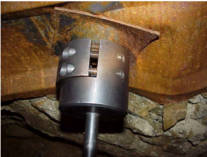
Figure 2.—Installation of pull claw on friction bolt.
