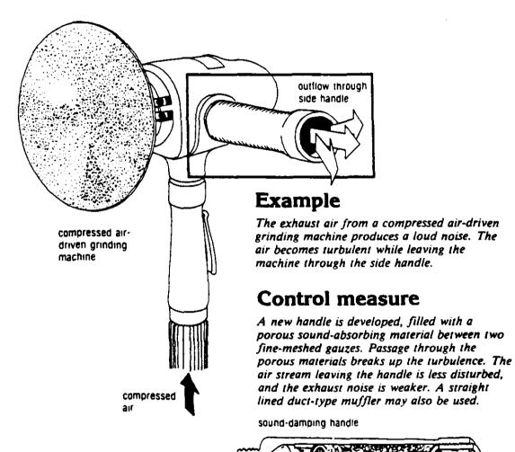
Reducing noise at the source: Installing a muffler (from <u>Noise Control</u>: A Guide for Workers and Employers, U.S. Dept. of Labor, OSHA).
