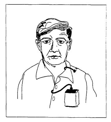
A noise dosimeter measures and stores sound energy over time. It can be worn in the pocket, as shown, or on the belt with the microphone positioned on the shoulder.
