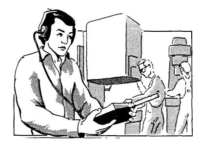
Measuring noise with a sound level meter (courtesy of Brüel and Kjaer Instruments).
