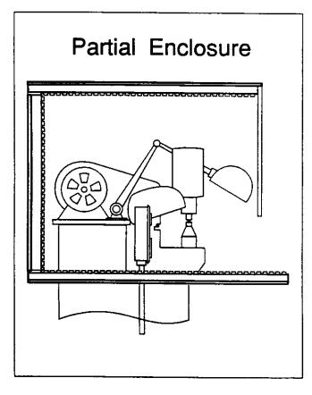
Interrupting the noise path with a partial machine enclosure (from <u>Noise Control</u>: A Guide for Workers and Employers, U.S. Dept. of Labor, OSHA).
