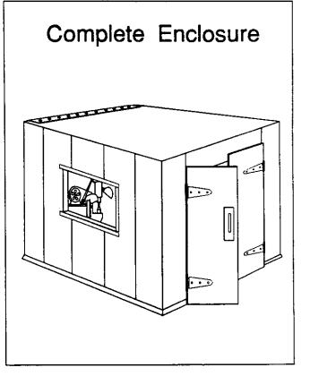
Interrupting the noise path using a complete enclosure.
