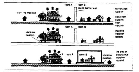
Reducing structure-borne vibration and reverberation (from <u>Noise Control</u>: A Guide for Workers and Employers, U.S. Dept. of Labor, OSHA).
