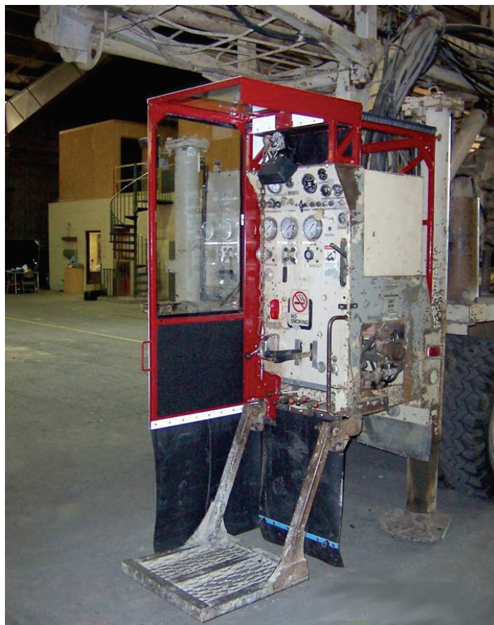
Figure 1.—The partial cab is retrofitted to the air rotary drill rig with a steel frame. The cab slides on a heavy-duty linear rail that supports the weight of the cab, allows for easy operation, and resists wear.
