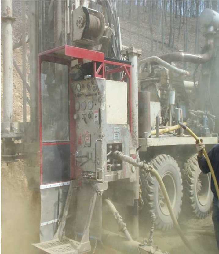
Figure 2.—In the field, the sound level at the operator's station without the partial cab was over 100 dB(A) during hammer drilling. The partial cab reduced the sound levels by 5–9 dB(A).
