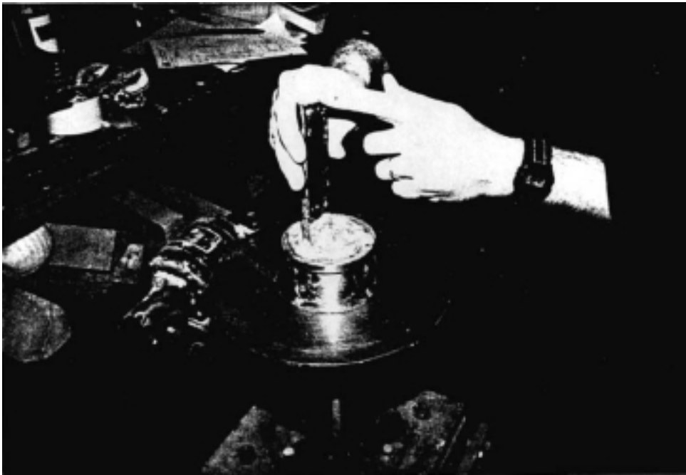
Figure 5.1. Mortar is tamped in the brass mold on the flow table.
