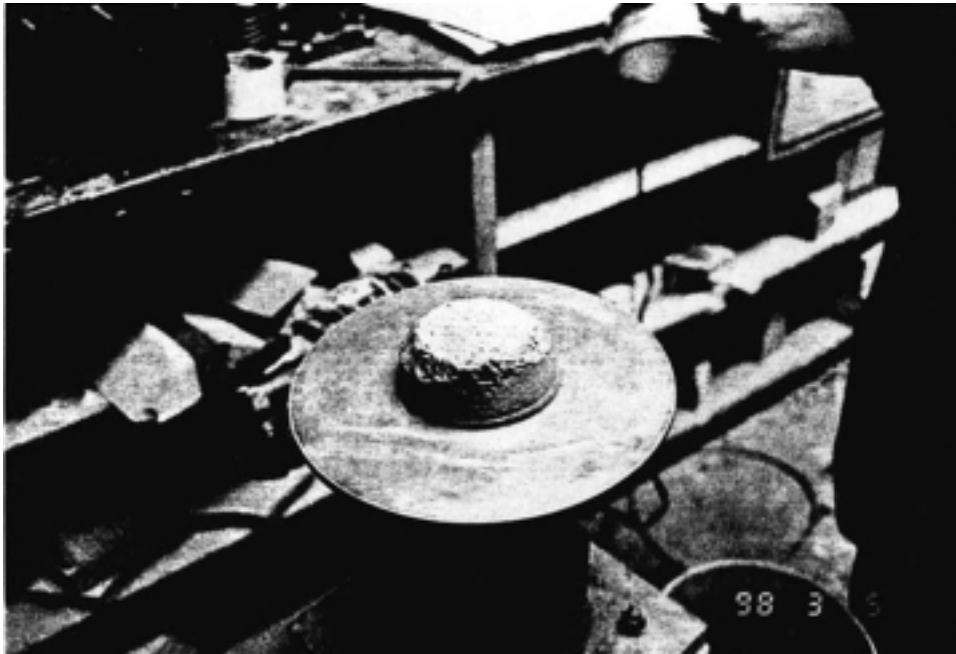
Figure 5.3. The brass mold has been removed from the mortar on the flow table.
