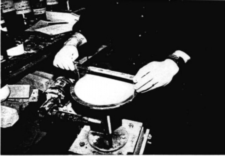
Figure 5.4. The diameter of the mortar pancake is measured with calipers.
