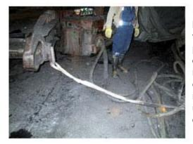
Undamaged trailing cables will isolate miners handling the cable from the hazardous voltages transmitted by the cable. To maintain this protection, the cable must be protected from damage and if it is damaged the damage must be readily detected and repaired. Small nicks and cuts in the cable can easily go undetected with most low- and medium- voltage power systems used today. These small nicks and cuts can expose miners to hazardous voltages.
