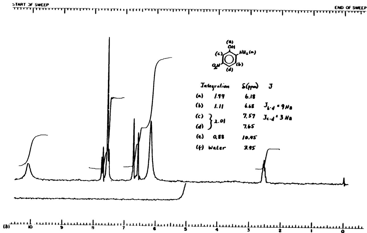
FIGURE 2. NUCLEAR MAGNETIC RESONANCE SPECTRUM OF 2-AMINO-5-NITROPHENOL (LOT NO. A8777)
