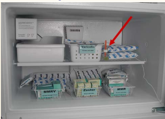
Fluid-filled biosafe liquid thermometer in freezer.
