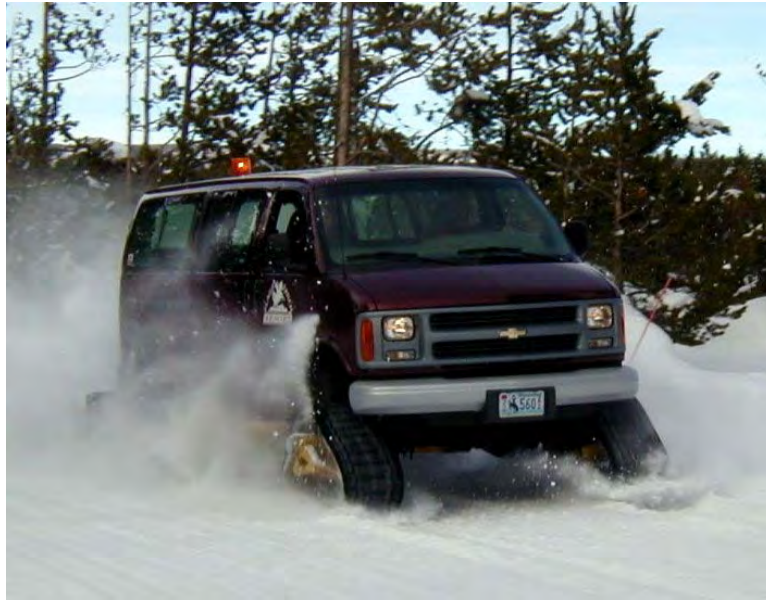
Figure 42: Conversion van snowcoach with Mattracks, Reference 9
