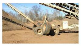
A crusher foreman was killed as he activated the stacker controls near the tandem wheels of a stacker conveyor while moving it with a front end loader. The stacker was connected to the loader with a chain. Even though the radial wheels were raised for moving, they contacted loose material which tightened the chain and nearly overturned the stacker that was still electrically energized and fully functional. The victim was attempting to raise the radial wheels higher to free them from the loose
