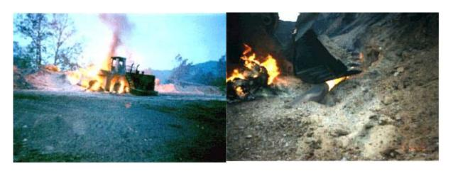
Recently, a fatal mining accident occurred when a front-end loader operator was removing material above a coal seam. The loader bucket penetrated a buried 20-inch diameter, high pressure, public utility natural gas transmission line. The loader became engulfed in flames resulting in fatal burns to the operator.
