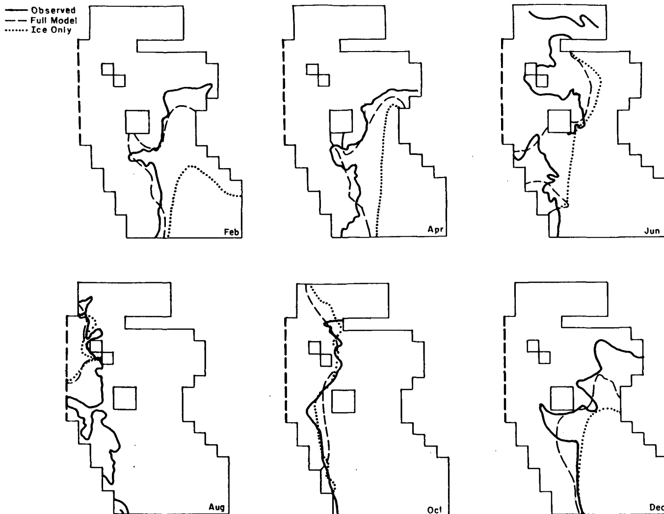
FIG. 15. Simulated and observed 50% concentration limits for both the coupled ice-ocean model and the ice-only model. The observed limits were taken from Fleet Weather (Suitland, Maryland, U.S. Navy) charts for 1979 at the end of the month.
