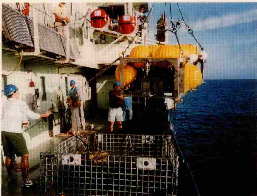
Experiment to measure vertical mixing of ocean waters was conducted by injecting SF_6 tracer into the Atlantic along a constant-density surface about 310 m deep. After six months the tracer had spread laterally over hundreds of kilometers, but vertically only a few tens of meters—much less than would be necessary to account for the vigor of the ocean's overturning. In this picture the SF_6 -injection sled is being retrieved aboard the R/V Oceanus, operated by Woods Hole Oceanographic Institution. (Courtesy of James Ledwell, Woods Hole.)
