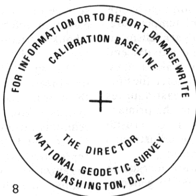
Figure 8.—Standard bronze marks of the National Ocean Survey/National Geodetic Survey.
