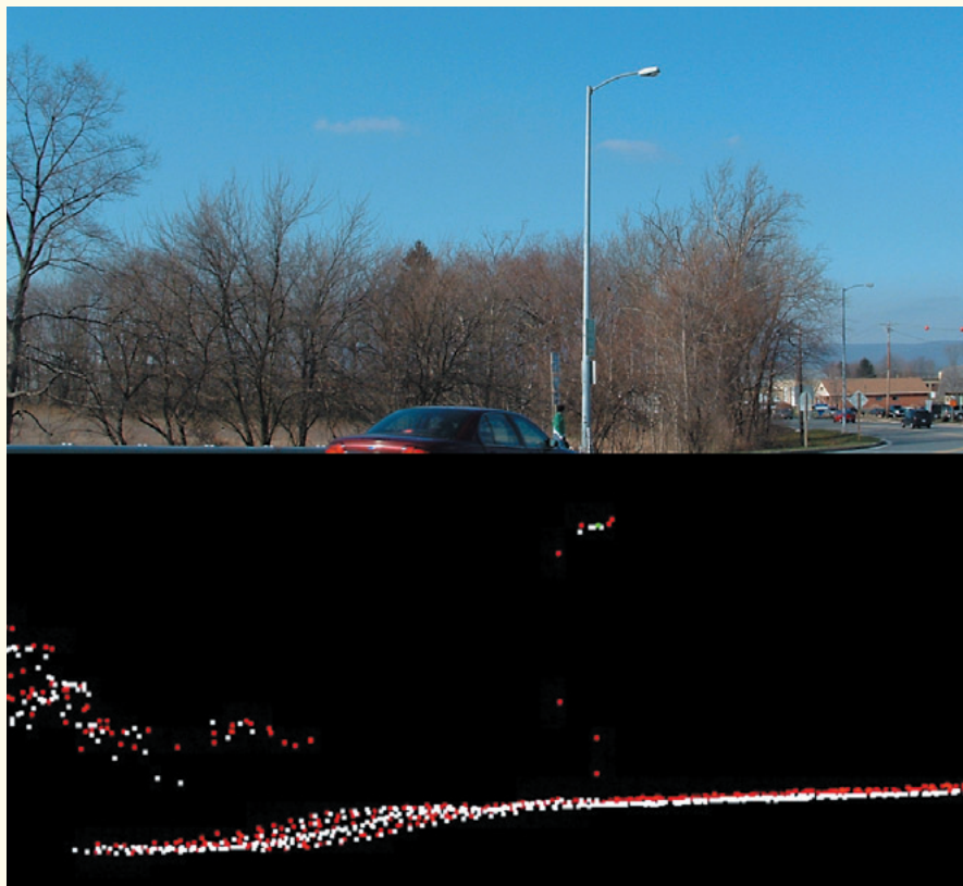
Figure 3 Photo of a light pole, one of the field-surveyed obstructions in the runway 5 approach at Frederick Municipal Airport. Bottom: a profile view of the corresponding LiDAR data points. The red dots represent the LiDAR data points from the tilted sensor, while the white dots represent the LiDAR data points from the nadir-pointing sensor. The green dot denotes the field-surveyed location.
