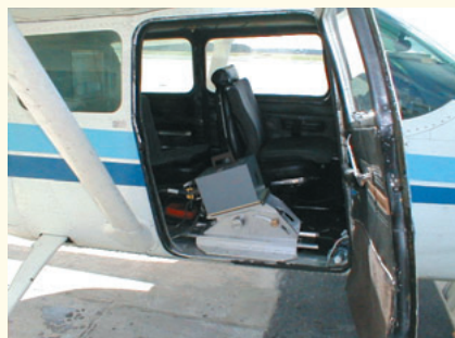
Figure 1 Custom sensor mount used in the 2002 study. This mount allows the lidar sensor head to be tilted between zero (nadir) and 40° forward. Here, the sensor head is shown in the 20° forward tilt position. The survey aircraft is a Cessna Skymaster.
