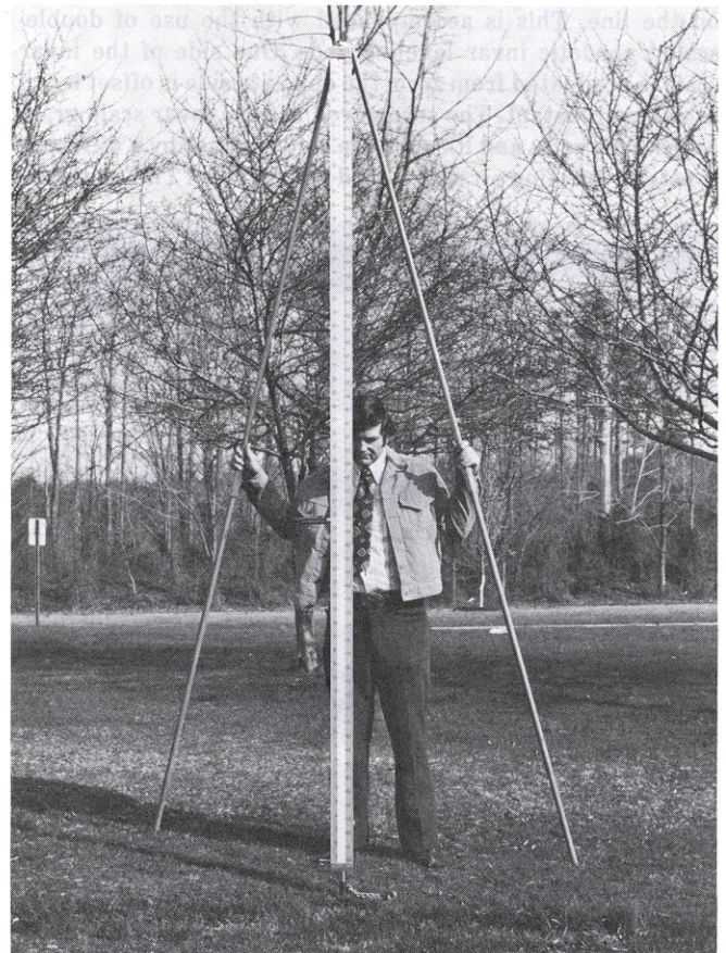
Figure 1. Geodetic level rod with brace poles.
