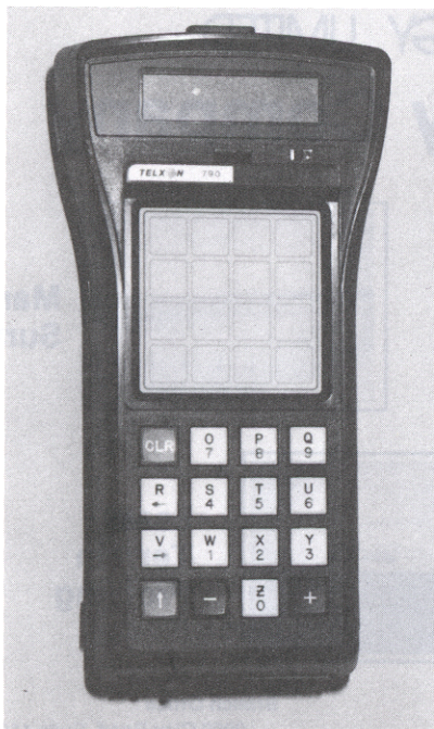
Figure 1. Programmable data-logger, data-storage device.
