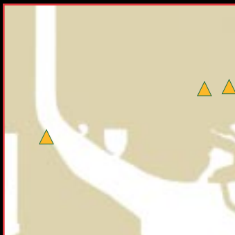
The first step in assembling a GIS involves creating a foundation "layer" of virtual geodetic control, shown above as ▲. These reference points serve as the basis – the "brass tacks" – for successive data layers, such as land and water boundaries.
