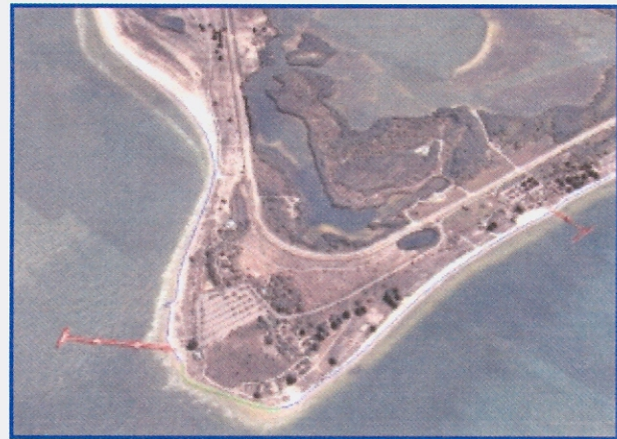
Figure 7: Feature-attributed LiDAR-derived shoreline and an orthophotograph draped over the LiDAR-derived DEM. Click on image to see enlarged.
