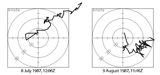
**Figure 19.** Hodographs (bottom 300 mbar) for 8 July 1987 (rain = 0.07 mm; strong low-level shear; CTP = 247 J/kg;  $HI_{low} = 11^{\circ}C$ ; soil moisture = 33%) and for 9 August 1987 (rain = 0.0 mm; strong low-level backing of the winds; CTP = -58 J/kg;  $HI_{low} = 9^{\circ}C$ ; soil moisture = 30%).
