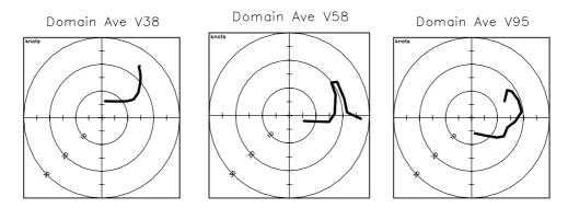
**Figure 10.** Hodographs to 300 mbar above ground surface (AGS) for three cases in the wet soil advantage regime where reduction of the initial and boundary winds increased the convective activity. In all three cases the winds back with height, and in all three cases, convective activity was greater in the reduced-winds runs than in the observed winds runs. See text for more information.
