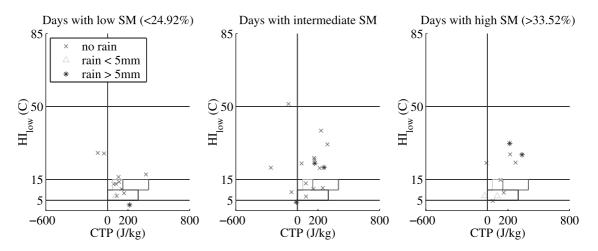
**Figure 15.** CTP,  $HI_{low}$ , and area-average rainfall for days with (left) low, (middle) intermediate, and (right) high soil moisture. Crosses indicate no rain, triangles indicate rain <5 mm, and stars indicate rain <5 mm.
