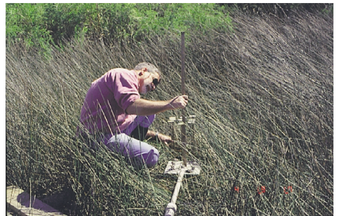
Measuring surface elevation at a Surface Elevation Table (SET) site in the high marsh
